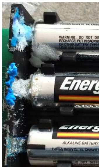
Figure 1: General Leakage Example (Not an Alcares Product)
